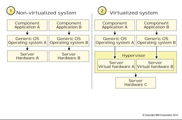
Figure 2-14. Comparing non-virtualized versus virtualized systems
