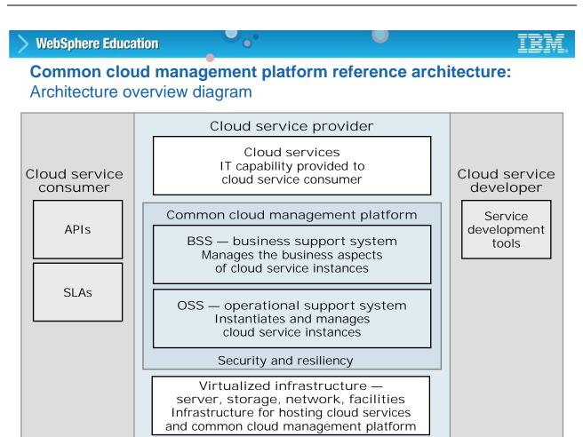
Figure 3-15. Common cloud management platform reference architecture: Architecture overview diagram
