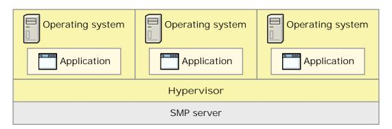
The figure shows one physical system with a type 1 hypervisor running directly on the system hardware, and three virtual systems using virtual resources provided by the hypervisor.
