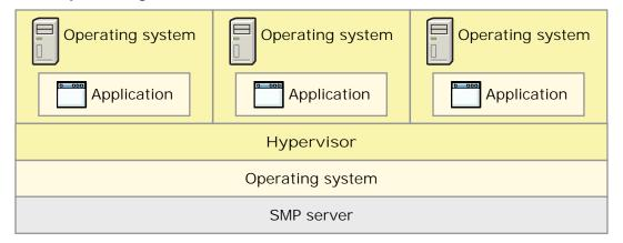
The figure shows one physical system with a type 2 hypervisor running on a host operating system and three virtual systems using the virtual resources provided by the hypervisor.
